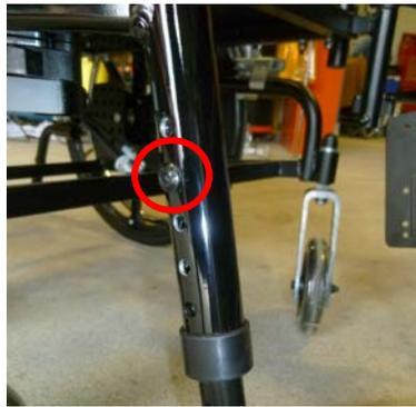
The foot plate can be moved fore and aft at the base of the leg rest, as well as adjusting the foot angle, using the same fastener set. The clamping mechanism has to be unbolted using a 10 mm wrench and an M4 hex key in order to reposition the plate placement fore and aft. The bolt and nut only need to be loosened to adjust the angle.
