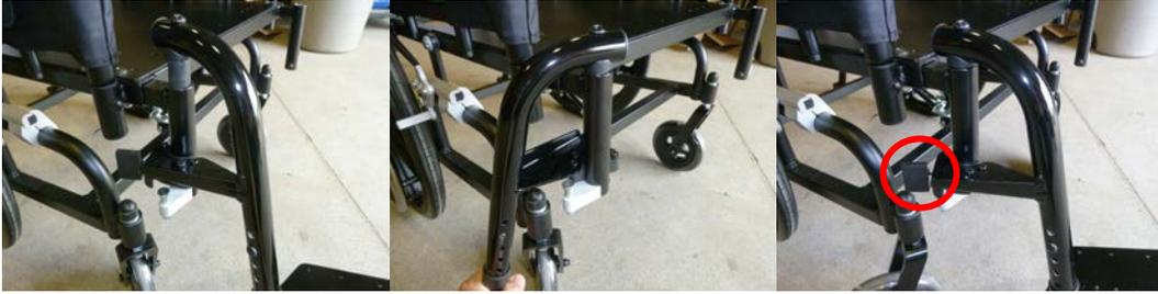
The leg rests can be adjusted to length using an M4 hex key. The bolt is removed and the length can be extended or shortened via sliding the lower tube inside the upper tube. There are various hole options to select from for reinserting the bolt.
