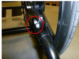
3. To remove the anti-tippers, the detent pin on the receiver can be disengaged and the anti-tippers slid out. The detent pin may be on the top or bottom, depending on how the receivers are mounted.
